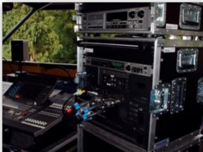
S-4000H Rack at FOH position
